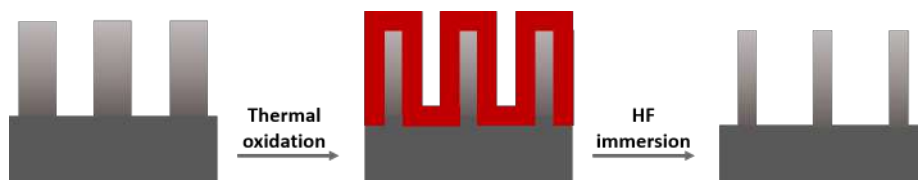
Figure 2.7. Increase of the pore diameter by oxidising and then removing the oxide layer by HF treatment.
