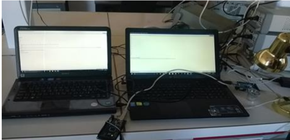
Fig. 3.24: Implementation of our text transmission system via visible light.
