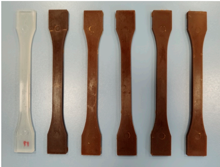
Figure 3. Visual aspect of the polylactide (PLA)/flaxseed flour (FSF) composite pieces processed with epoxidized linseed oil (ELO) and maleinized linseed oil (MLO) corresponding, from left to right, to: PLA, PLA/FSF, PLA/FSF + 2.5ELO, PLA/FSF + 5ELO, PLA/FSF + 2.5MLO, and PLA/FSF + 5MLO.
