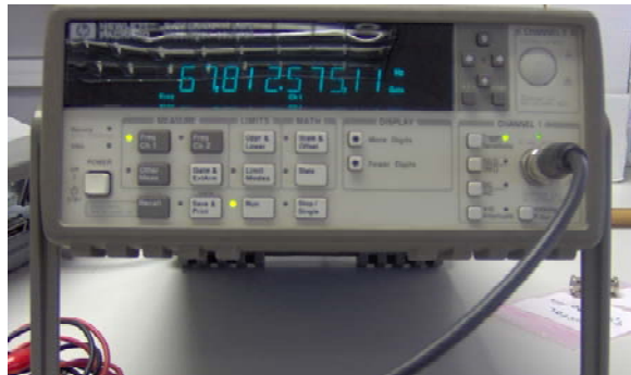
Fig. 4.18. Frequency meter HP 53181A employed in the experimentation.
