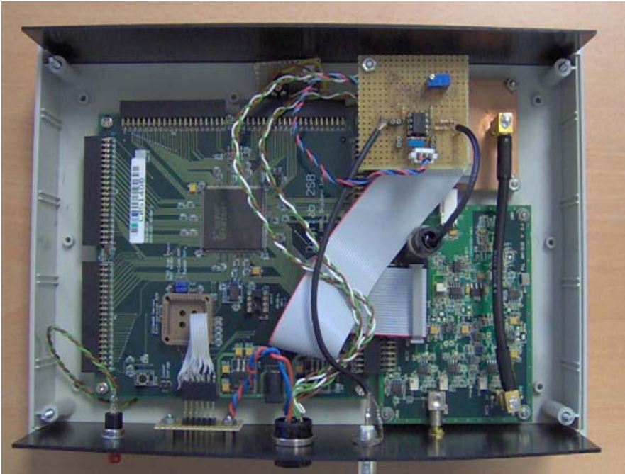
Fig. 3.25. Photo of the A-d PLL complete system assembled.
