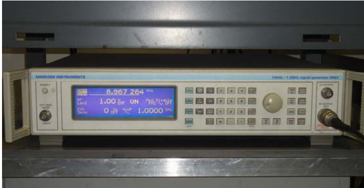
Fig. 4.19. Signal generator Marconi 2023 employed in the experimentation.
