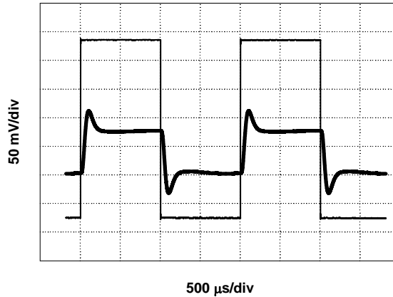
Fig. 5.5. Preliminary step response of the system,—Modulating Signal, — Step Response. Adapted from [Torres06-2].
