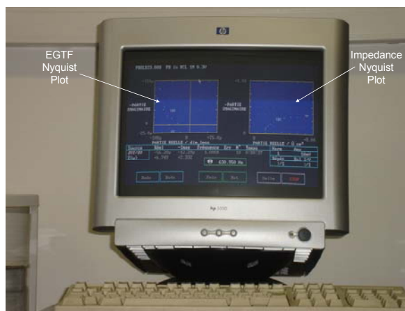
Fig. 4.16. Measurer software in the PC connected to the TFA.
