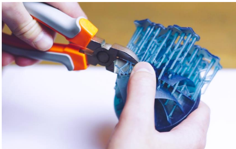
Picture 15. Removing the supports
