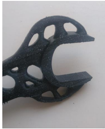
Picture 71. Rounded connections improve the quality of the part
