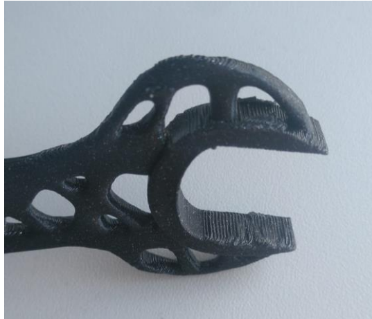
Picture 58. Low quality of the connections and rough surface in the mouth
