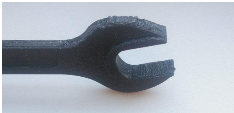
Picture 39. Surface rough of the mouth of the vertical orientation part
