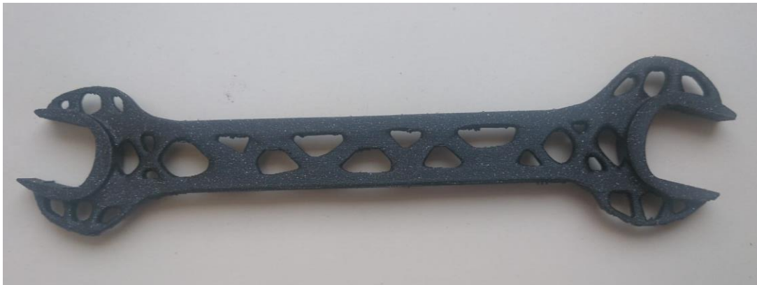
Picture 69. Surface smooth of the horizontal orientation part
