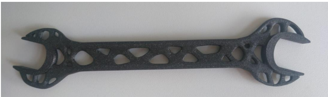
Picture 56. Surface smooth of the horizontal orientation part
