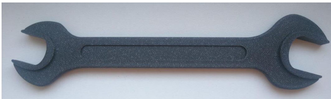
Picture 37. Surface smooth of the horizontal orientation part
