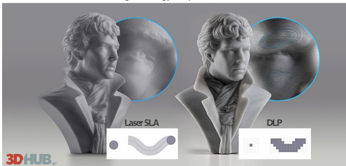
3D Printing Technology Comparison: SLA vs. DLP
