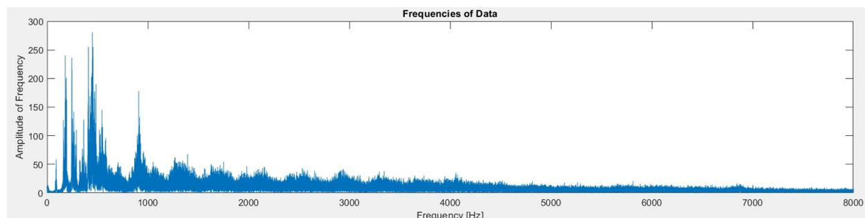
*Fig. 26 FFT results of data from microphone 2*
