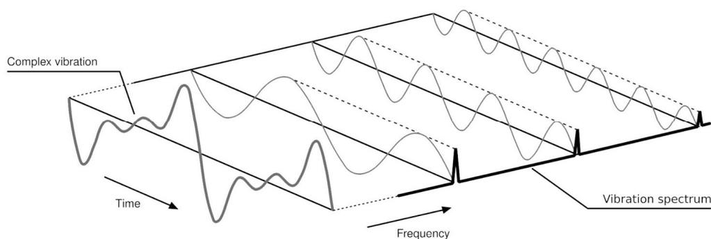
*Fig. 22 FFT processing of a complex signal (Power-MI, n.d.)*
