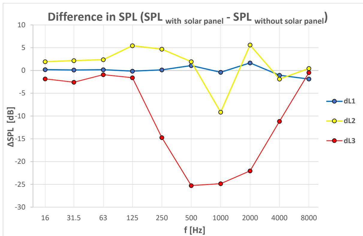
Fig. 19  $\Delta$ SPL plot for the solar panel
