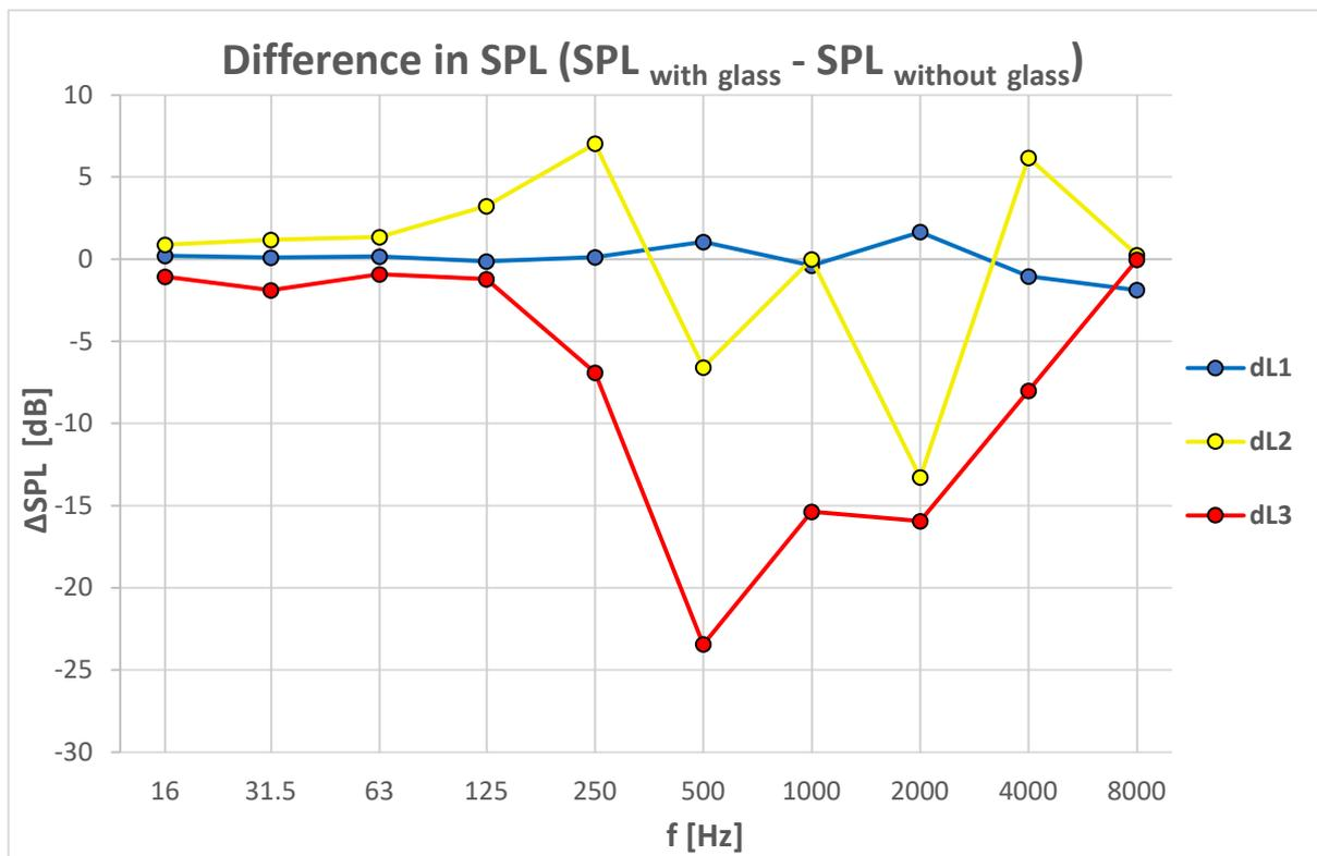
Fig. 18  $\Delta$ SPL plot for glass
