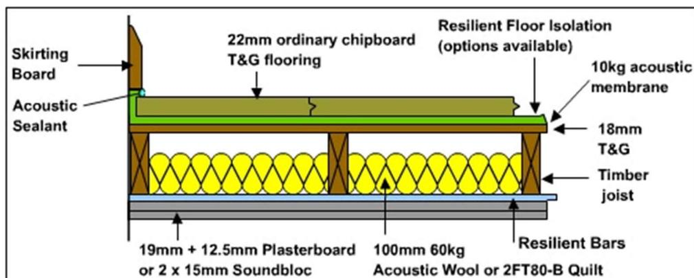
*Fig. 21 Diagram of a floating floor
