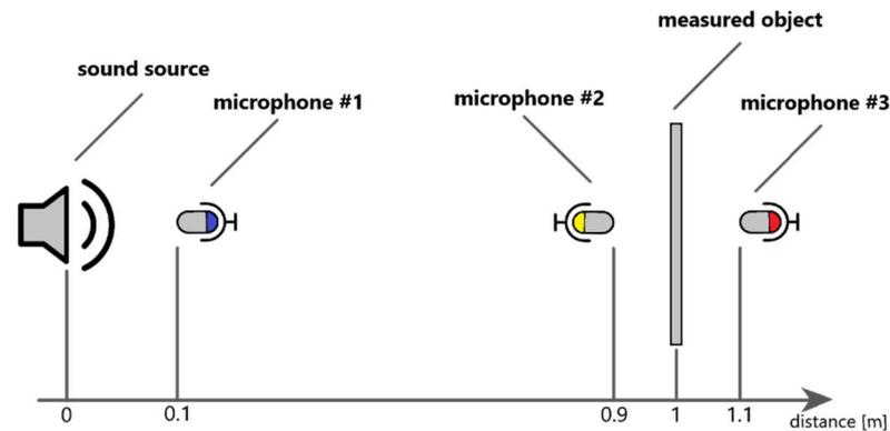
*Fig. 13 Measurement setup's schematic diagram*
