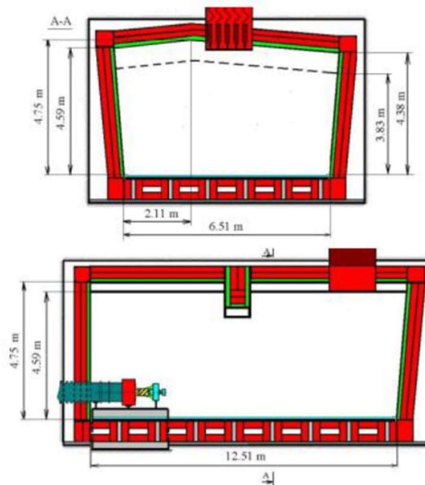
*Fig. 8 Vertical cross-sections of the chamber
