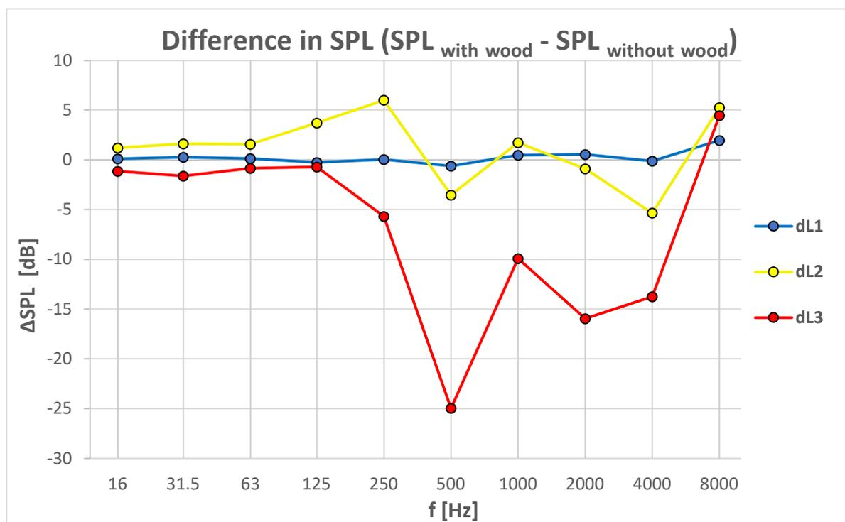
Fig. 16  $\Delta$ SPL plot for wood
