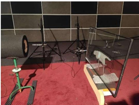
*Fig. 14 Photo of the measurement setup from the session with a glass window*
