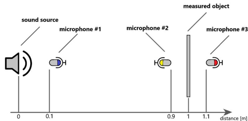
*Fig. 13 Measurement setup's schematic diagram*
