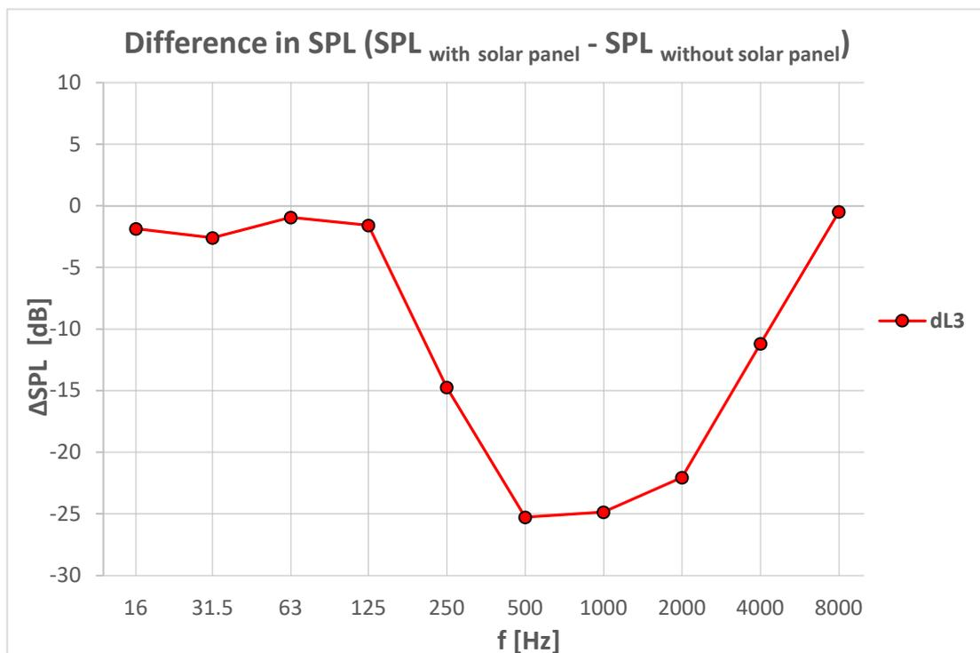
Fig. 32 ΔSPL plot for the solar panel - L3 microphone only
