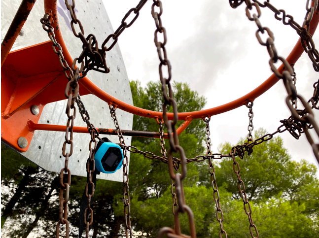
Figure 6.11: Net sensor placed behind the net.
