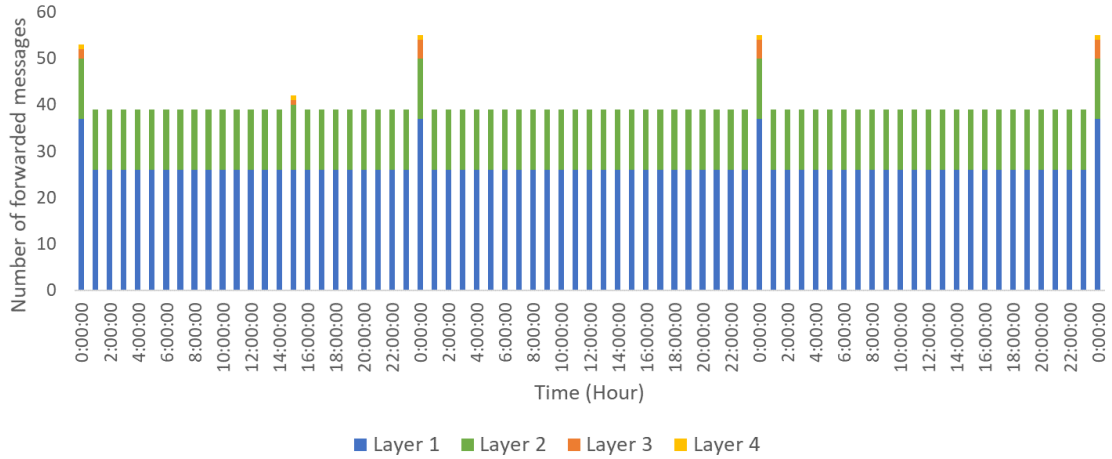
Figure 6.11. Number of messages forwarded by each layer at the Regular Farmer Mode.
