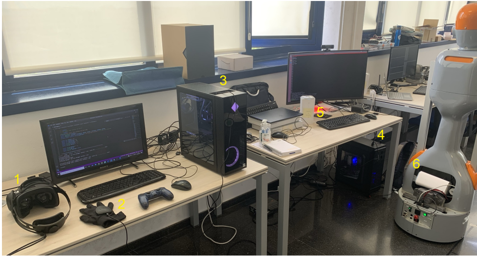
Figure 3.11: (1) Varjo XR-3, (2) Sensorial XR, (3) Windows PC, (4) Linux Server, (5)(6) Modems
