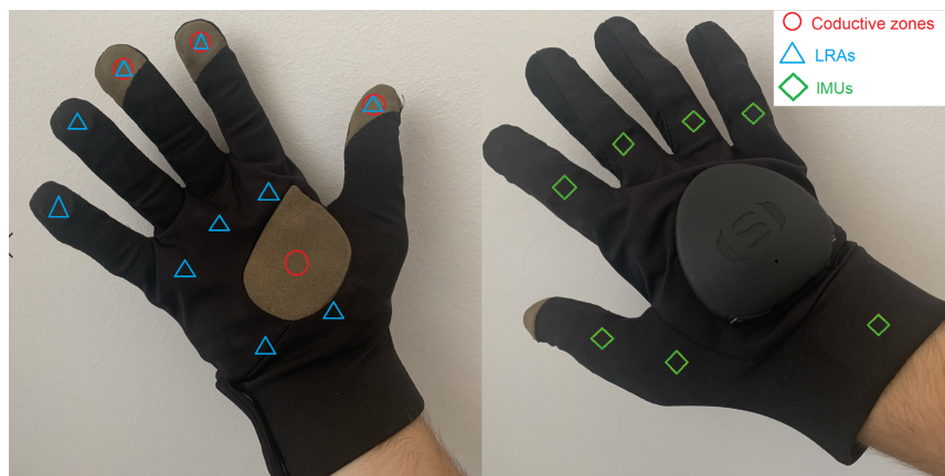
Figure 3.5: Sensorial XR in detail
