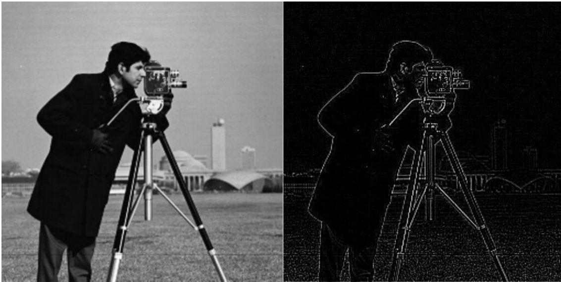
Figure 2.3: Edge detection example with Laplacian filter.
