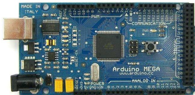
Figura 9: Arduino Mega
