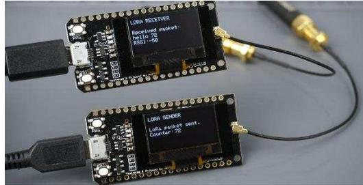
Figura 10: TTGO LoRa 32 OLED V1 [10]
