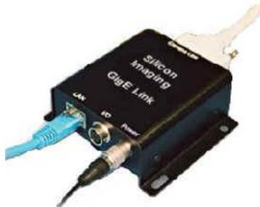
Figura 2.4. Módulo GigE-CameraLink, interface Ethernet 10/100/1000
