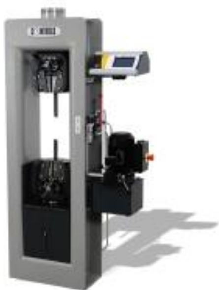
Figura 34. Semi-Automatic 500/1000 KN testing machine. Fuente: [18]
