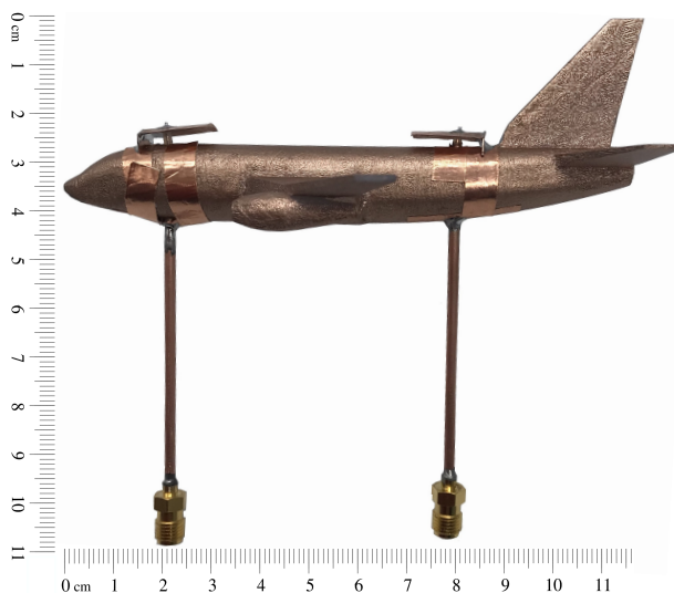
Figure 6.31: The manufactured prototype of a scaled Boeing 737 airplane, excited by 2 pifa antennas.
