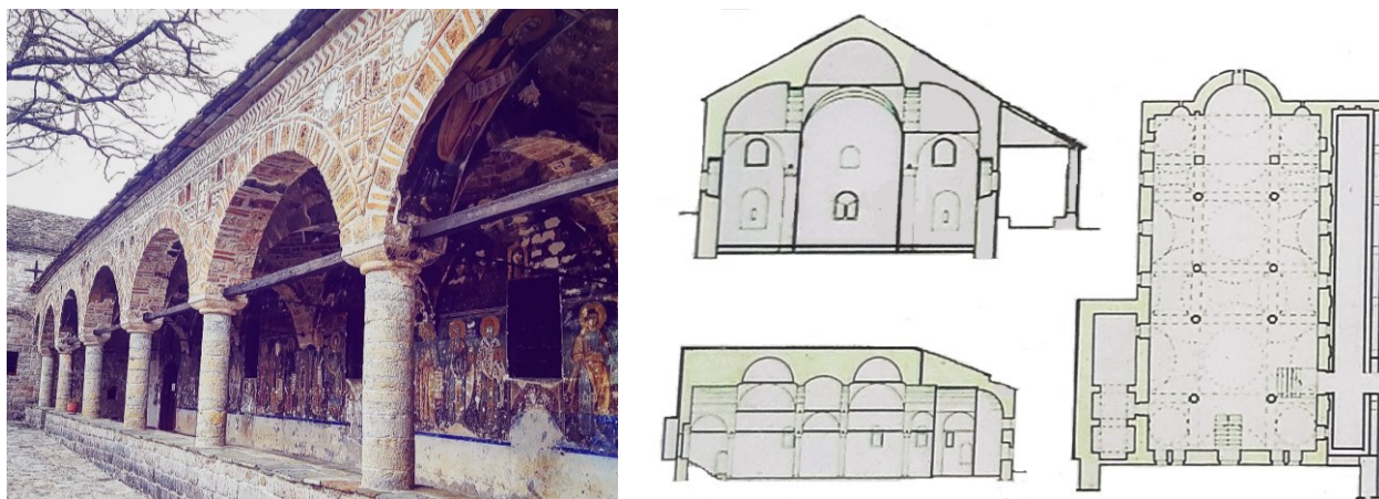
Figure II.5 A. View of the open porch of the church of St. Nicholas ; B. Plan, longitudinal and transverse sections of the church of the Holy Mother of God , both in Moskopole (Albania).
