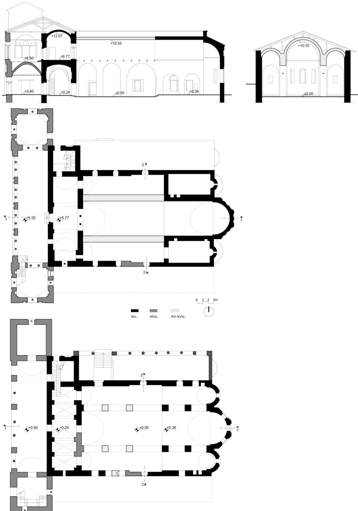
Figure I.25 St. Sophia in Ohrid, after the Ottoman reconstruction. Ground floor plan ( \pm 0.00 ); gallery plan (+6.50); longitudinal section (1-1) and transversal section (2-2).
