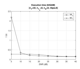
Figure 9: Average computing times (seconds) in Setup 4 (experiment with 10000 channel matrices).
