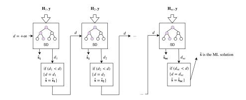
Figure 2: Procedure of sequential detection with adjustable radius.
