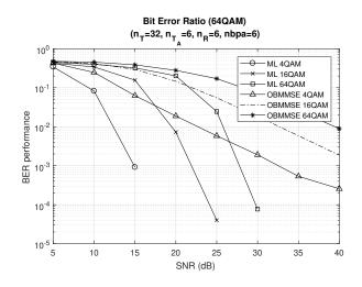
Figure 4: BER comparison between OB-MMSE (non-ML method) and the proposed ML methods
