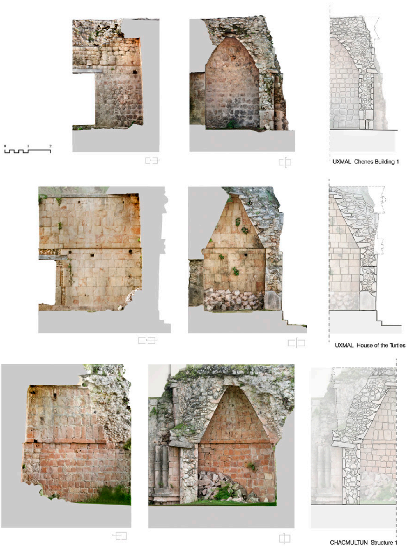
Fig. 11: Comparative orthophotos and sections obtained from the photogrammetric models of three of the vaults studied
