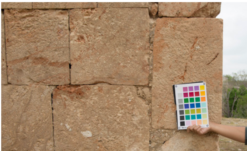
Fig. 9: Use of a colorchecker when performing a digital photogrammetric survey
