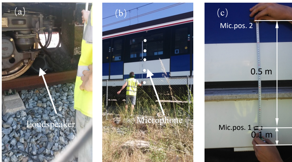
Figure 20. Measurements of sound pressure on a stationary train. (a) Loudspeaker location, (b) microphone positions, (c) separation of microphones.
