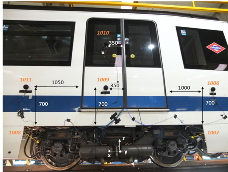
Figure 22. Field measurement positions used to measure sound distribution on the train outside surface.
