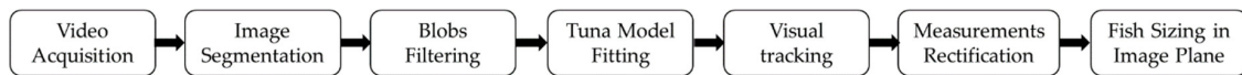
Figure 6. Sequence of video processing algorithms involved in the process of fish sizing.
