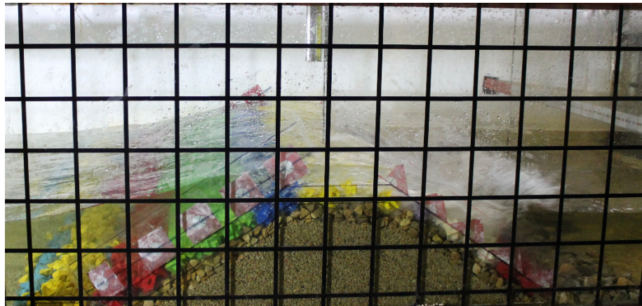
238 239 Fig. 6. Visual inspection of the overtopping layer thickness (OLT) during the physical tests.
