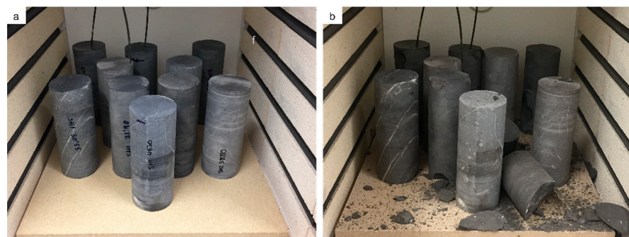
Figure 8. Samples before (a) and after (b) heated to 600 °C. Effects of temperature involve visible fissure growth, splitting, and cracking.
