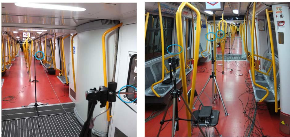
Figure 3. Overview of interior noise measurements on a running metro vehicle.
