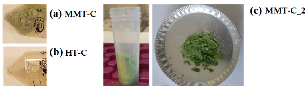
Figure 3. Visual appearance of chlorophyll hybrid nanopigments obtained with MMT (MMT-C) (a), HT (HT-C) (b) and MMT with a higher chlorophyll dye (CD) concentration (MMT-C_2) (c).
