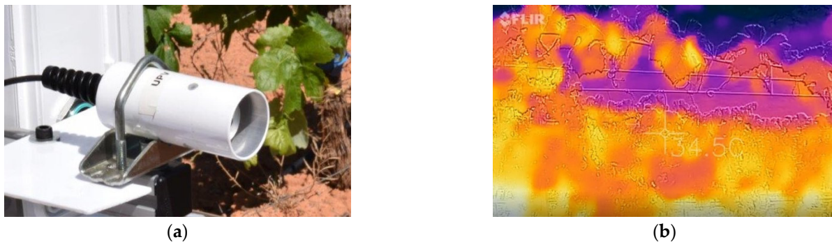
Figure 6. Non-invasive monitoring of canopy temperature: (a) infrared radiometer (Apogee Instruments, Inc., Logan, UT, USA); and (b) thermographic images of a vineyard from a terrestrial vehicle (FLIR Systems, Inc., Wilsonville, OR, USA).
