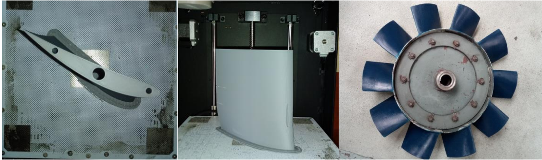
Fig. 5. 3D printouts of fan blades with space for reinforcing bars, the fan modified by adding prints changing the shape of the blades [11]
