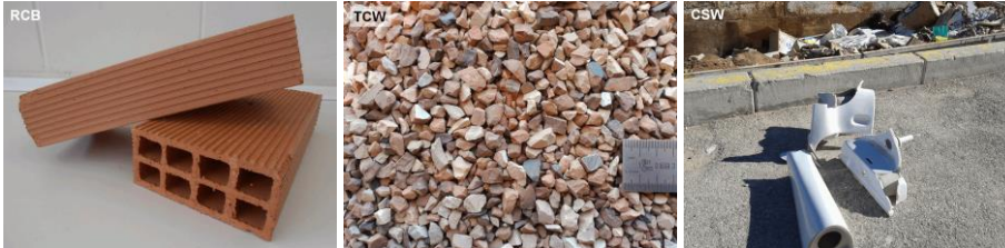
Figure 1. The original RCB, TCW and CSW ceramic waste materials
