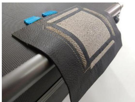
**Figure 9.** Flexible 3D Boosted sensor manufactured.
