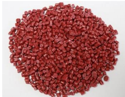
Figure 2.23: Pellets of recycled HDPE [34]
