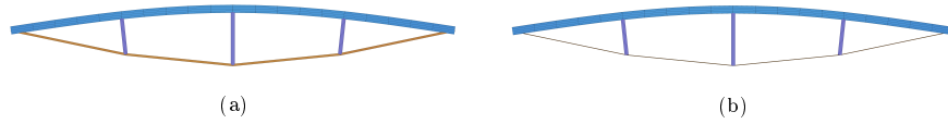
Figure 3: Configurations with the same rod slenderness \bar{\lambda} = 1.5 and different cable-rod slenderness ratios: a) \bar{\lambda}_c/\bar{\lambda} = 5 and b) \bar{\lambda}_c/\bar{\lambda} = 15
