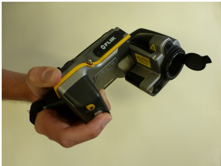
Fig. 5.8. Infrared camera “FLIR B 335” (done by J.C.C and R.F.P.)
