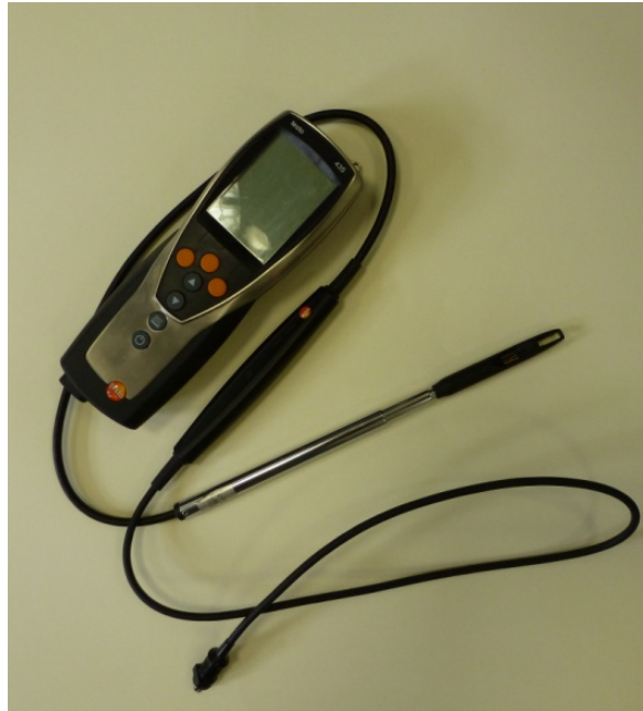
Fig. 5.6. Multi-functional measuring instrument “TESTO 435” (done by J.C.C and R.F.P)
