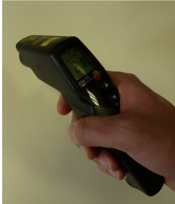
Fig. 5.5. Infrared thermometer “TESTO 830” (done by J.C.C. and R.F.P.)
