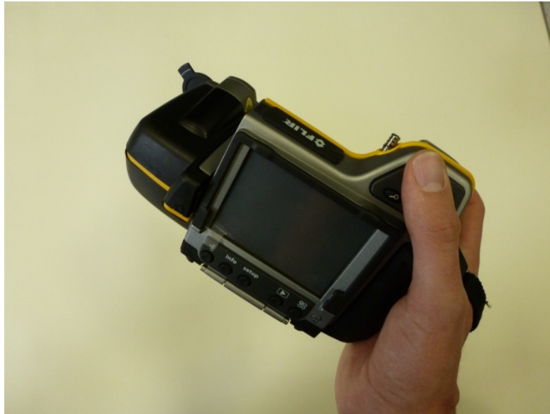
Fig. 5.7. Infrared camera “FLIR B 335” (done by J.C.C and R.F.P.)
