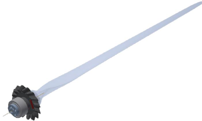
Figure 4.1: Assembled Blade. From left to right, the blade shaft (2.2) with the two 6180 bearings inserted; the bevel gear (2.3) in black with the Hall Magnet and the Blade profile
