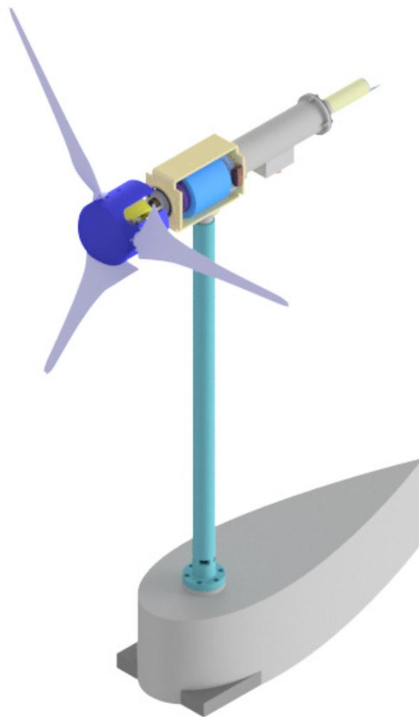
Figure 3.11: G06 turbine setup for the Wind tunnel experiment with NACA0030 dummy printed in 3D
