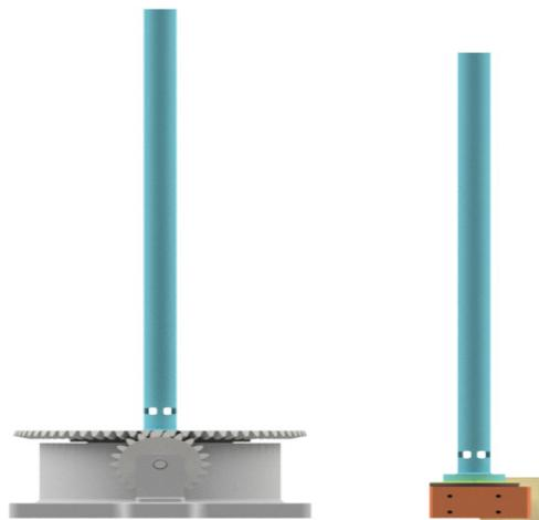
Figure 3.4: Size comparison Handmade Rotatory stage vs RT2A075
