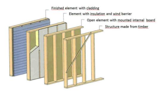
Figure 55 Construction of timber façade <sup>[17]</sup>
