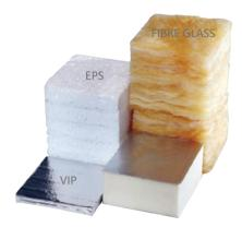
Figure 45 Traditional insulation materials vs VIPs [24]
