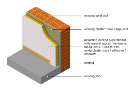
Figure 47 Plasterboard laminated fixed to the existing wall <sup>[13]</sup>
