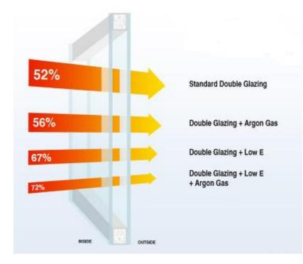
Figure 57 Heat loss reduction according to the method <sup>[30]</sup>
