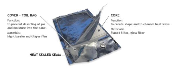
Figure 44 Vacuum insulated panel composition [23]
