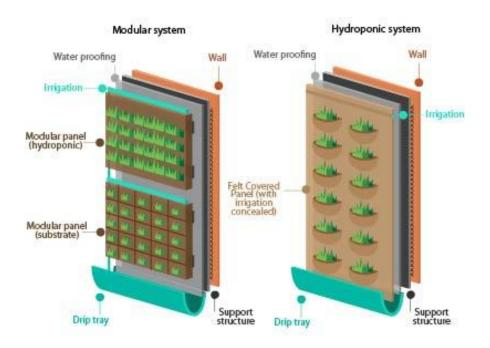
Figure 46 Two general types of green wall systems; modular and hydroponic <sup>[12]</sup>
