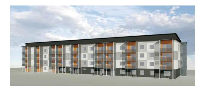
Fig. 8 Building after full renovation with TES facade, new balconies and new tilted roof (source: arch. Kimmo Lylykangas)
