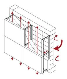
Figure 42 Thermal behaviour in winter <sup>[22]</sup>
