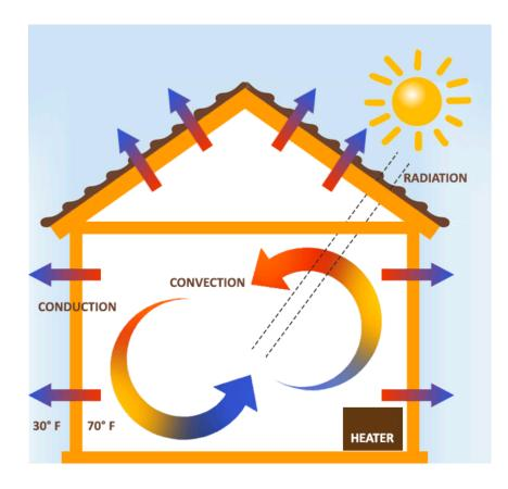
Figure 39 The idea of radiation, conduction and conversion [44]
