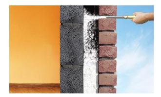
Figure 50 Cavity wall Insulation with blown mineral wool <sup>[25]</sup>
