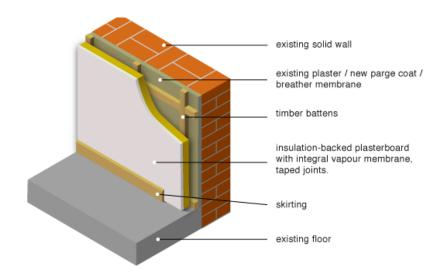
Figure 48 Insulation boards fixed to the wall timber battens and covered with plasterboard <sup>[13]</sup>
