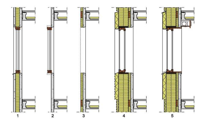
Fig. 7 Phases of full renovation with TES facade elements (source: arch. Kimmo Lylykangas)
