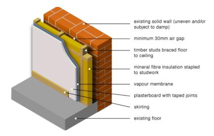
Figure 49 Insulation fixed to a freestanding studwork <sup>[13]</sup>
