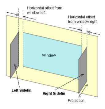
Figure 62 Local shading – sidefins [18]
