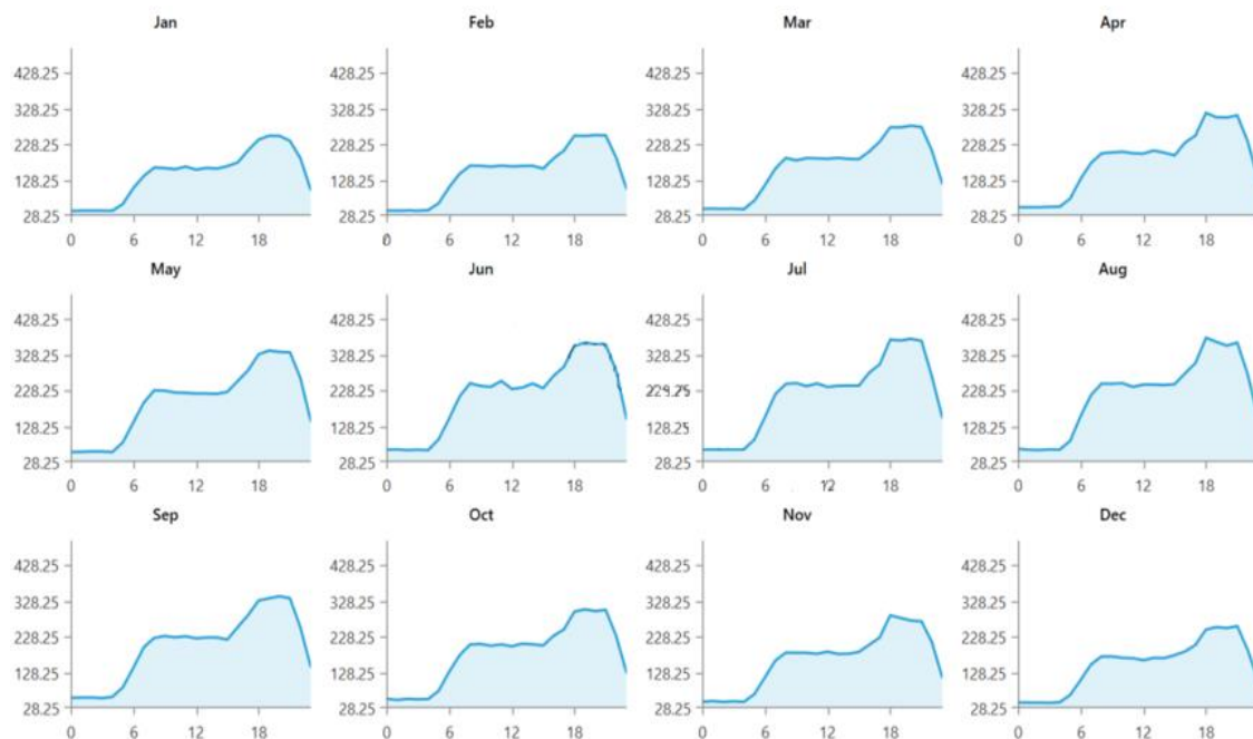
Figure 3.2: Monthly average of electric load variation of the SWRO desalination plant. Load demand in kW (X-axis) and hours per day (Y-Axis). Simulated in HOMER Pro™.
