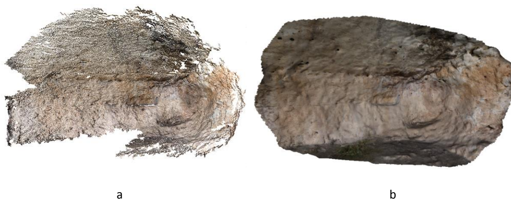
Figure 2.3. The interior of a shelter: a) 3D point cloud; b) photorealistic 3D model.
