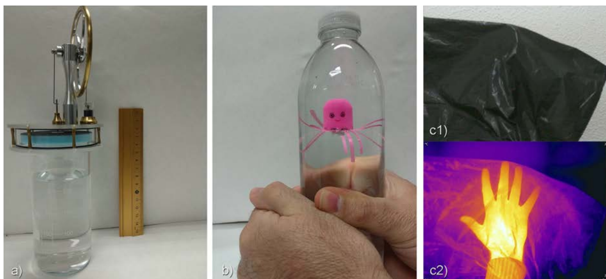
Figure 1. Images of assemblies for three energy-related experiments: a) The Stirling Engine. b) Diving with jellyfishes. c) A hand covered with a trash bag: c1) Visible light image; c2) Infrared thermal image.
