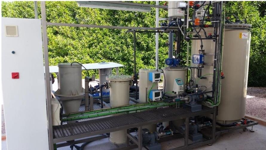
*Figure 3.7. AnMBR<sub>AD</sub> pilot plant.*
