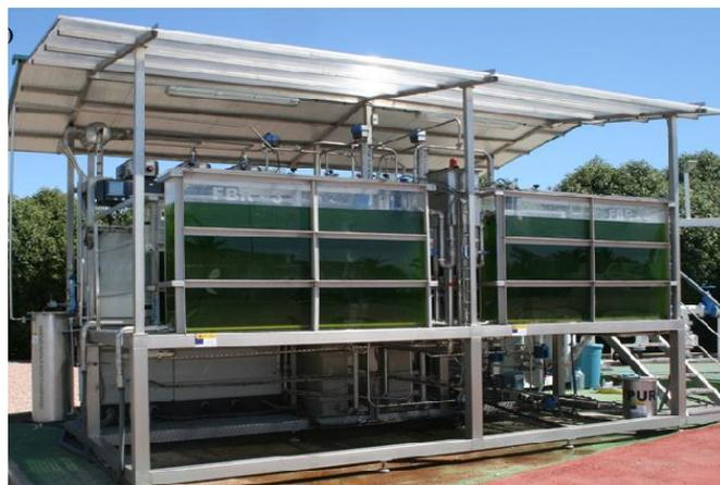
*Figure 3.6. MPBR pilot plant.*
