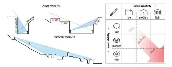
Fig. 2 | Visibility of photovoltaic surfaces from public spaces (close visibility) and from hills (remote visibility); criticity matrix and gradient (diagram: M. C. Munari Probst & C. Roecker).
