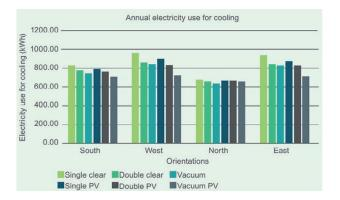
**Fig. 8** | Annual cooling electricity consumption with different types of glazing in Hong Kong (source: YANG Hongxing).
