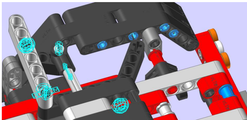
Figure 123. LTM_42043-2 > Self-aligned "JA" > A detail of the joint between truck and trailer in Recurdyn.
