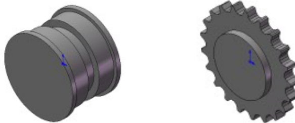
Figure 65. Predetermined single flange (left ) and sprocket (right) in Recurdyn's toolkit "Chains".
