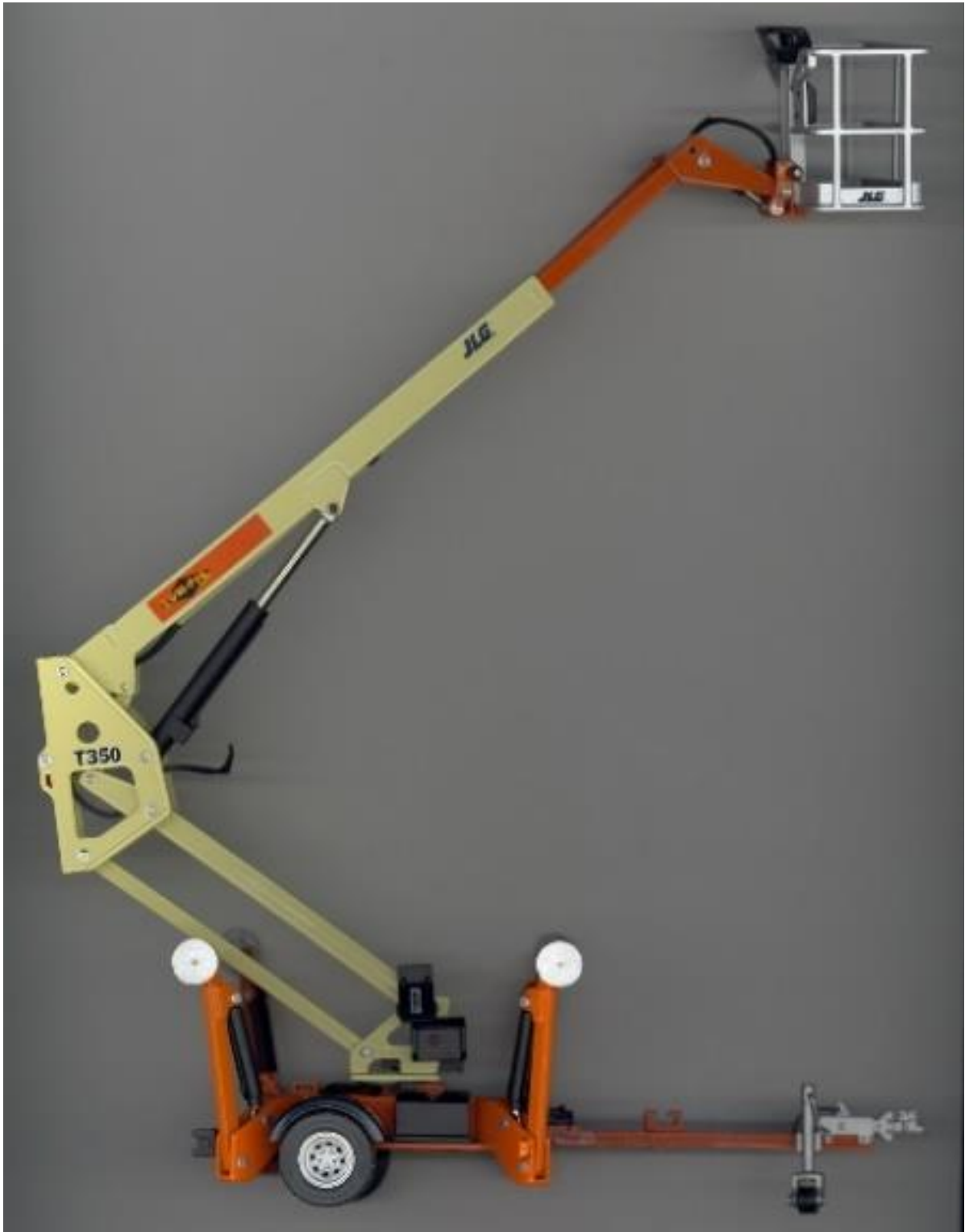
Figure 56. A machine to work at height: T350 elevator. Source: http://www.upv.es/vltmodels/10-c33-obras-pub-r.html .
