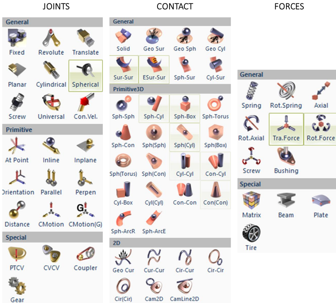
Figure 33. All types of joints, contacts, and forces available in RecurDyn.
