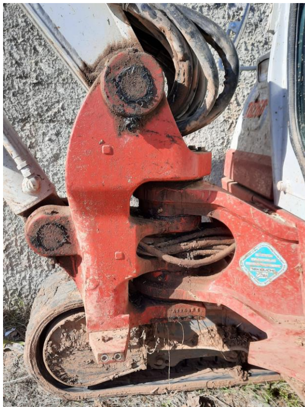
Figure 206. LTM_8047-1 > A real life machine (4/11). > Rotation of shovel with respect to cabin's chassis.
