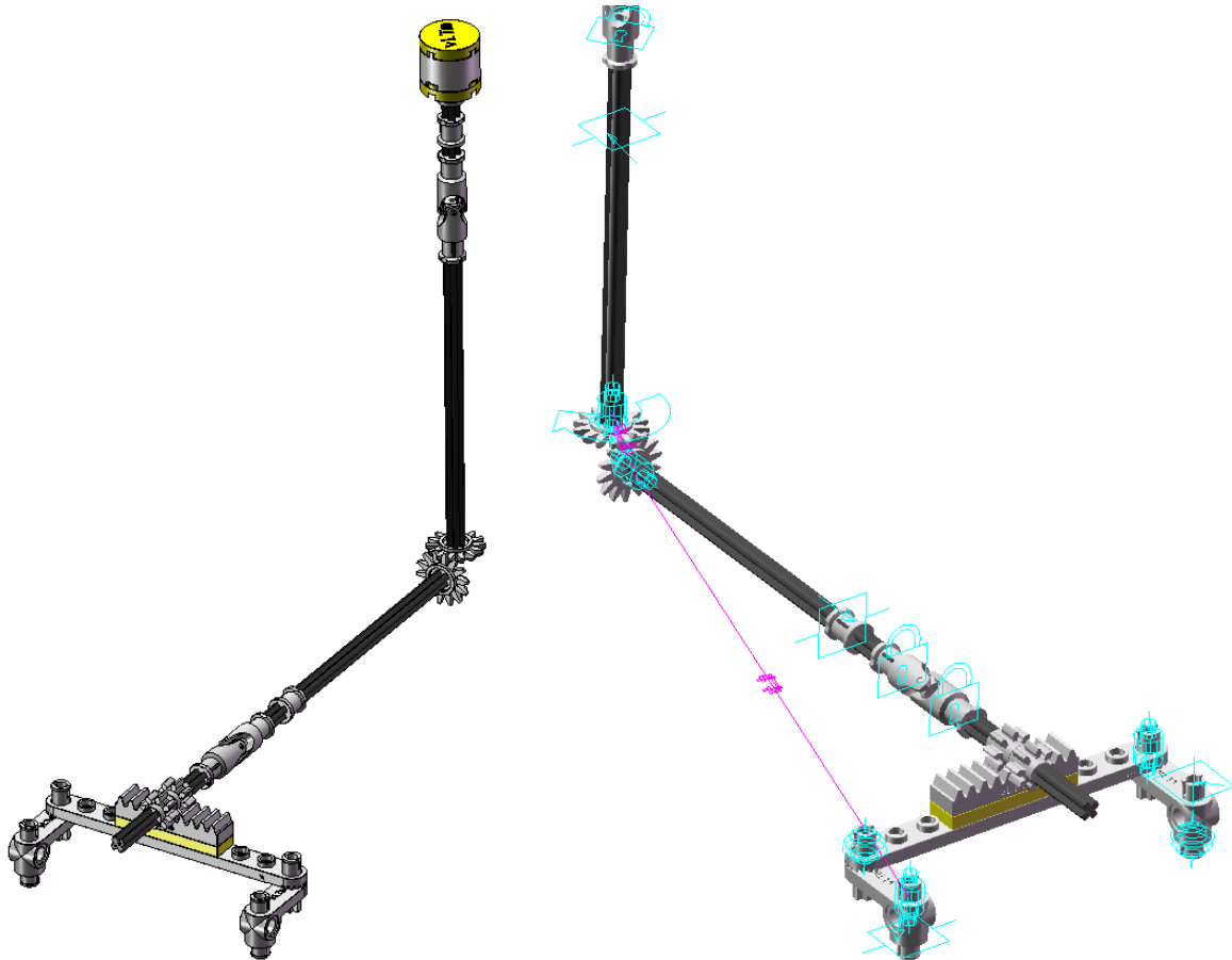
Figure 182 LTM_8862 > Self-aligned Mechanism "Direction" (D) in SolidWorks® 2007 (left) and in COSMOSMotion 2007 (right). 1 DOF to be controlled to move the vehicle to the left or to the right. FTTG: 001.
