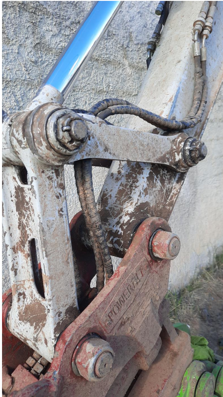
Figure 210. LTM_8047-1 > A real life machine (7/11). > The 4-bar used to control the inclination of basket with respect to chassis of the cylinders. It is a planar mechanism.
