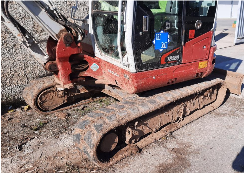
Figure 205. LTM_8047-1 > A real life machine (3/11). > Rotation of shovel with respect to cabin's chassis, rotation of cabin's chassis with respect to chains' chassis, and chains.
