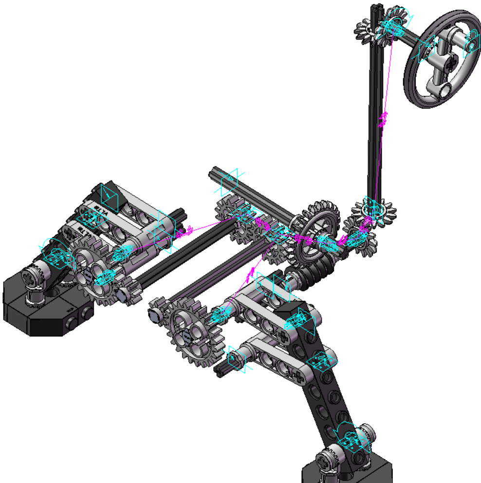
Figure 187. LTM_8862 > Self-aligned "U" in COSMOSMotion 2007. 1 DOF to be controlled: to extend or to contact the supports.
