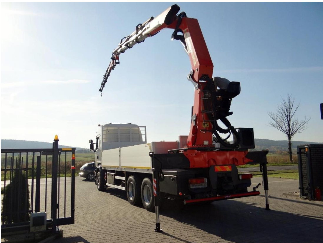
Figure 110. LTM_42043-2 > A real life machine (#3 > 2/2): SCANIA R 480 / 6X4 / HDS PALFINGER PK 40002 + FLY JIB. Source: this is the source (matysek.pl/en)
