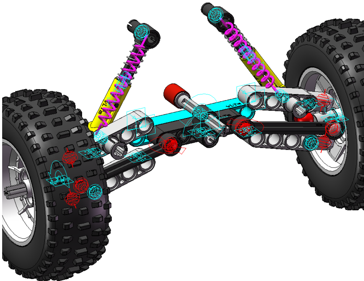
Figure 234. LTm_42124-1 > Self-aligned "D" in COSMOSMotion 2007. 5 DOF: 2 independent shock absorbers and 2 wheels (4 passive DOF) and left-right control (1 DOF to be controlled).
