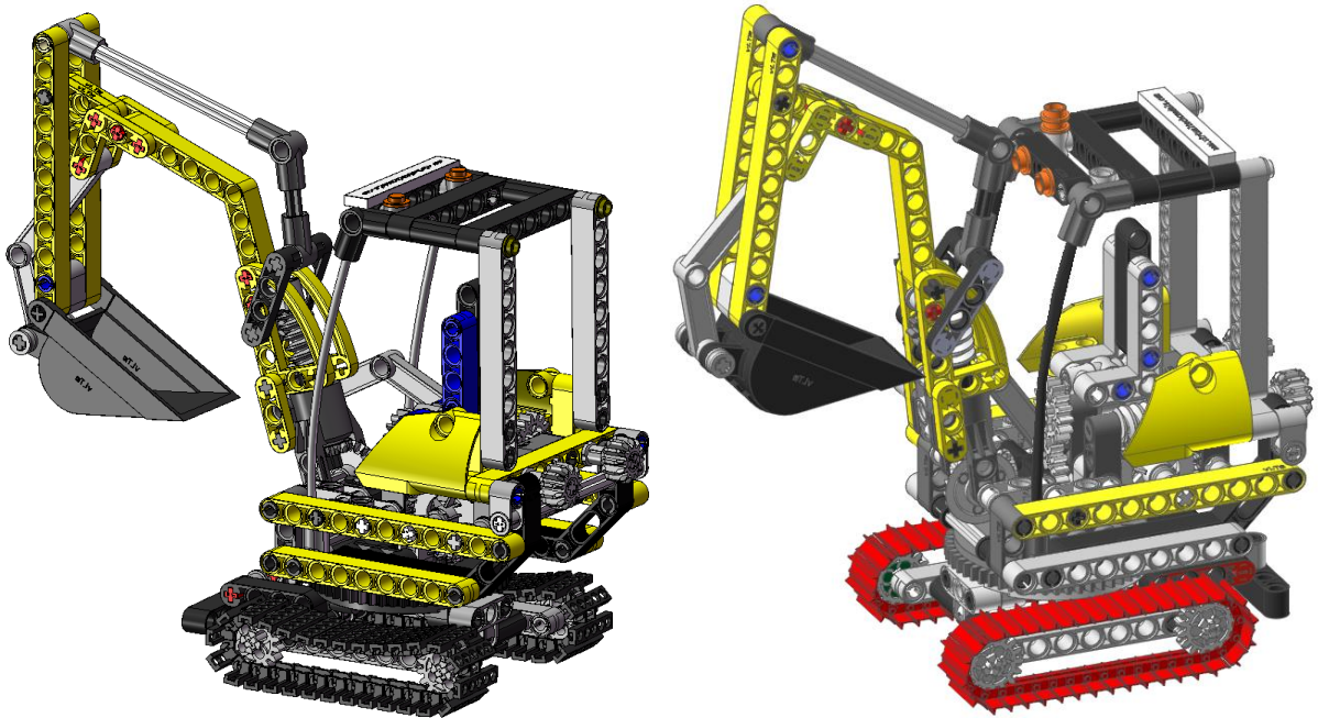
Figure 200. LTM_8047-1 in SolidWorks® 2020 with original chains (left), and after creating chains with the “Track_LM” toolkit in Recurdyn (right).
