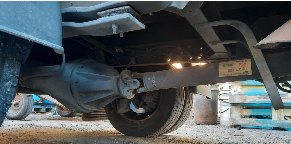
Figure 146. LTM_42043-2 >"P"> An example of the differential and the universal joint (2/2).
