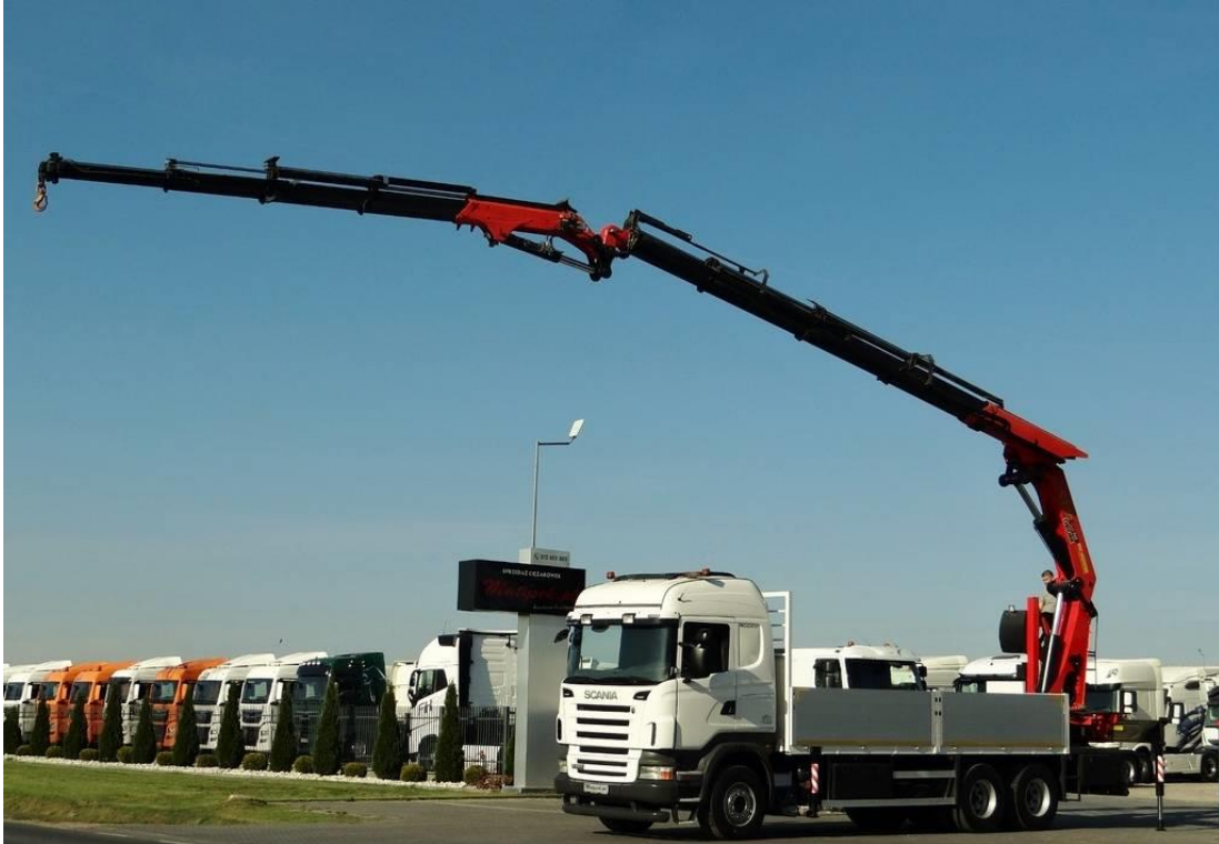
Figure 109. LTM_42043-2 > A real life machine (#3 > 1/2): SCANIA R 480 / 6X4 / HDS PALFINGER PK 40002 + FLY JIB. Source: this is the source (matysek.pl/en)
