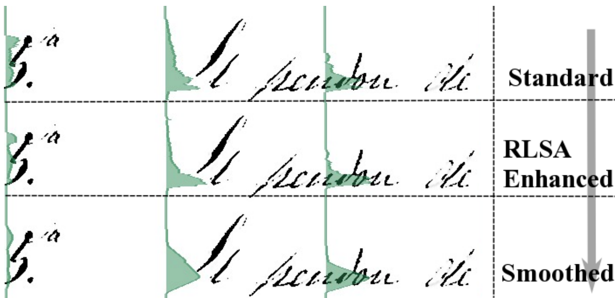
Figure 3.12: View of the impact of the RLSA and rolling median filter on the vertical projection profile calculation of a sample line.
