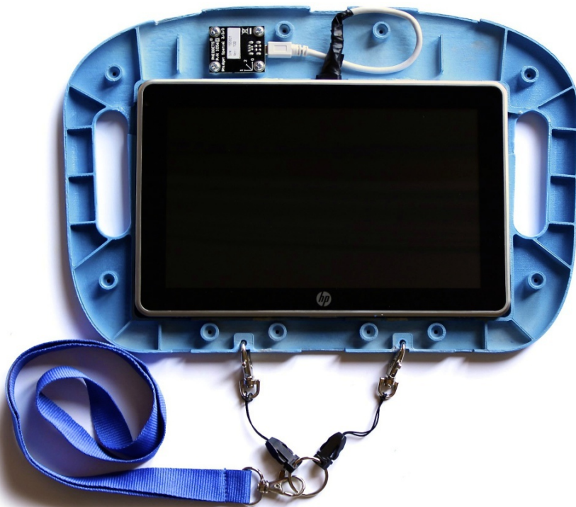
Figure 3.6: Internal view of the case built, with the Tablet PC, the USB accelerometer and the neck ribbon.
