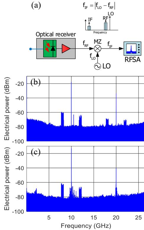
Figure 3. (a) Down-conversion scheme and electrical spectra (16-QAM data signal of 500 MHz bandwidth is transmitted), (b) System A with down-converted Qbias modulated signal, and (c) System B with down-converted CS modulated signal. LO: local oscillator, MZ: mixer, RFSA: RF spectrum analyzer.
