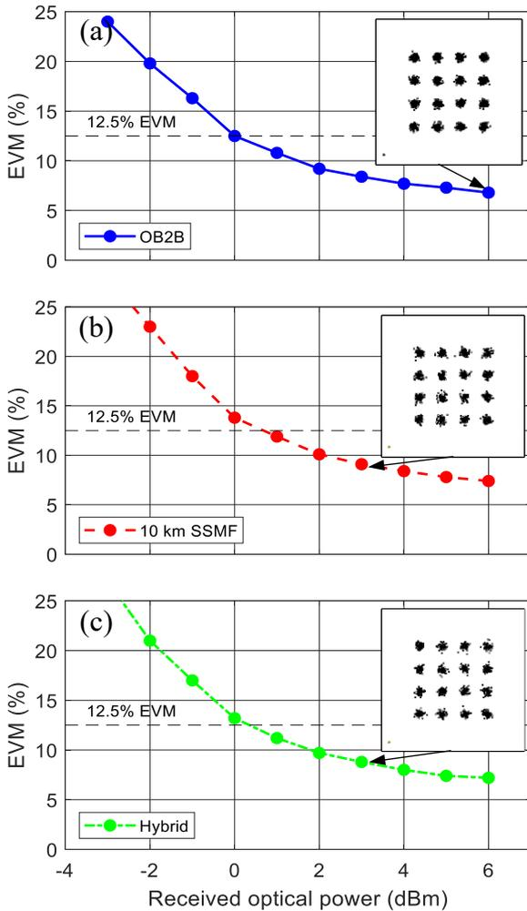
Figure 5. EVM performance of the System B transmitting a 16-QAM data signal with 500 MHz bandwidth for: (a) OB2B, (b) 10 km SSMF, and (c) full hybrid link with 10 km SSMF and 1.5 m long FSO channel. Insets show the constellations.
