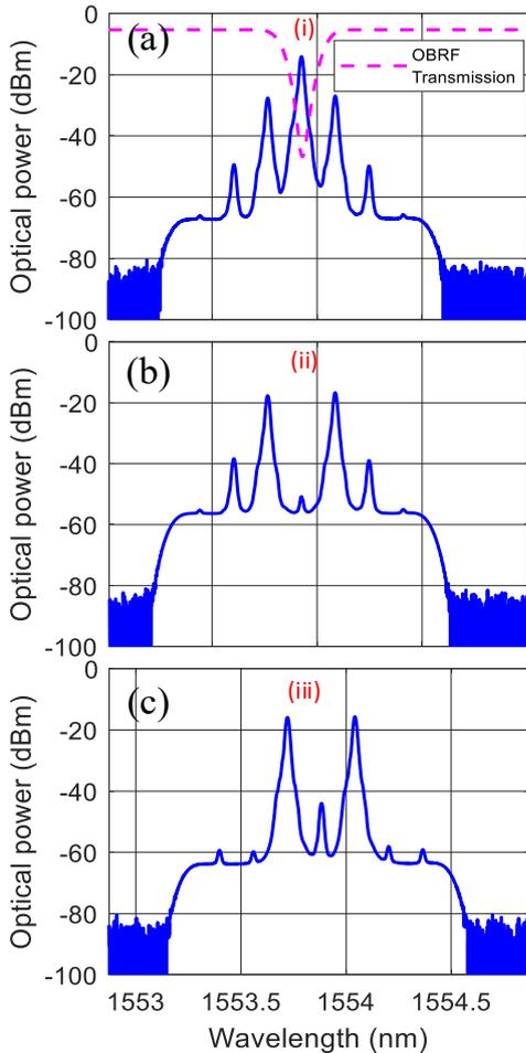
Figure 2. Optical spectra of: (a) Quadrature bias modulated signal (System A) before OBRF, (b) Quadrature bias modulated signal (System A) after OBRF, and (c) Carrier suppressed modulated signal (System B).
