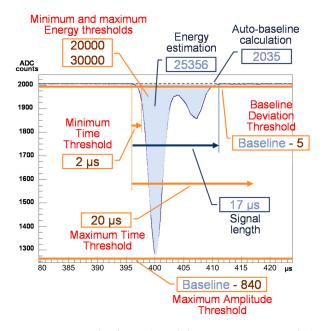
**Figure 5.** Example of signal candidate generation. In red, the complete set of configuration parameters to generate an event candidate from a PMT signal. In blue, data estimated by the event processor over the reconstructed signal by the BLR algorithm.
