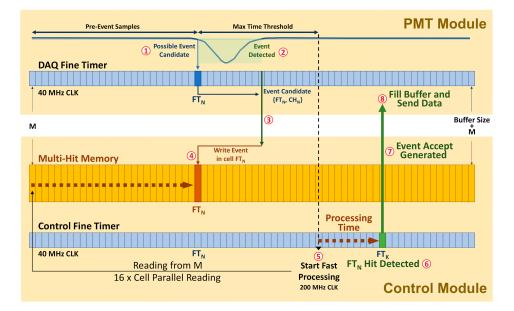
Figure 9. System event detection and Multi-Hit Memory scheme and functionality example.
