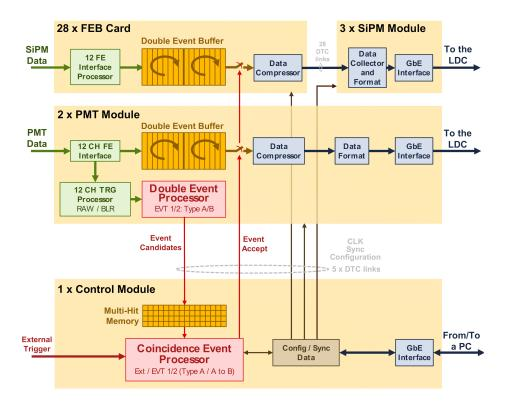
Figure 4. NEXT-DEMO trigger scheme.
