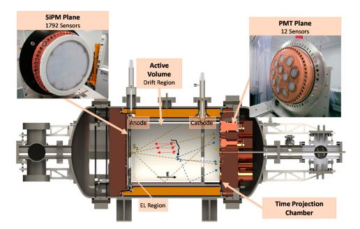
**Figure 1.** Schematic view of the NEXT-White Detector. Top right: Picture of the PMT sensors plane. Top left: Picture of the SiPM sensors plane. In the active volume of the TPC: Drawing with the principle of operation of the detector.
