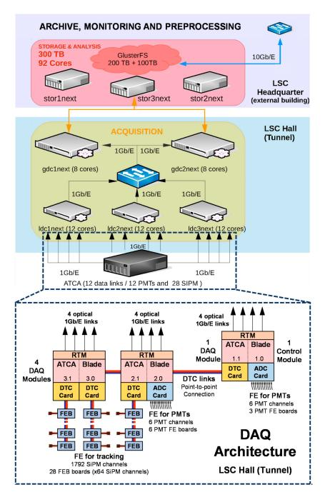
Figure 3. NEXT-White Data Acquisition Hardware Architecture.
