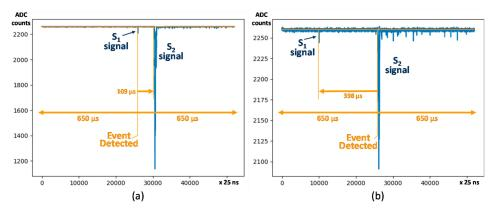
**Figure 2.** NEXT-White most common signal searches: (**a**) Online  $S_1$  signal search, with offline  $S_2$  signal search; (**b**) Online  $S_2$  signal search with offline  $S_1$  signal search. In both cases, a data acquisition window of 1300 µs and pre-trigger of 650 µs is applied.
