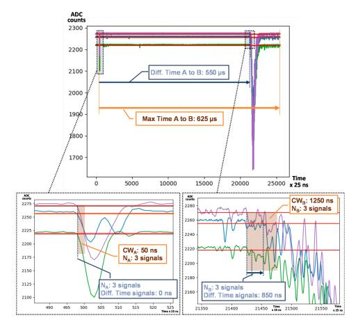
**Figure 8.** Event Accept example in Double Searching Mode: Run 4405 electron like Type A signal followed by a Type B signal for PMT0, PMT1 and PMT2. Double Search configuration set: 625  $\mu$ s Maximum Time Event A to B. Type A signal configuration set: 50 ns Coincidence Window (CW<sub>A</sub>) and 3 minimum number of PMT hits (N<sub>A</sub>). Type B signal configuration set: 1250 ns Coincidence Window (CW<sub>B</sub>) and 3 minimum number of PMT hits (N<sub>B</sub>).
