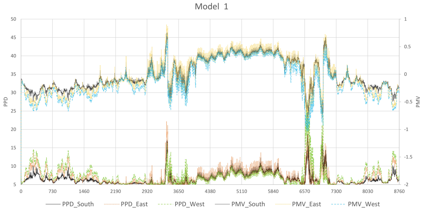
Figure 4. PPD and PMV values for Model 1 in different areas (south, east, and west).
