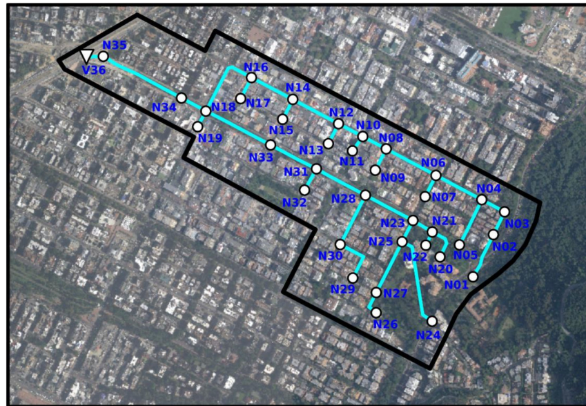
Figure 5. Representation of the E-Chico network in the Storm Water Management Model (SWMM) model. (Background image taken from [31]).
