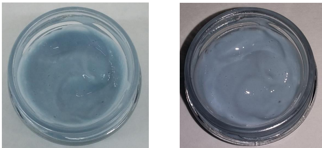
Figure 57. Printing paste with embedded C-phycoerythrin, based on conventional synthetic components(left) and natural commercial alternative printing paste (right)
