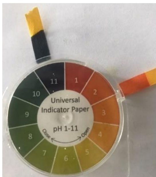
Figure 101. Validating the pH of the treatment solutions with pH indicator test paper
