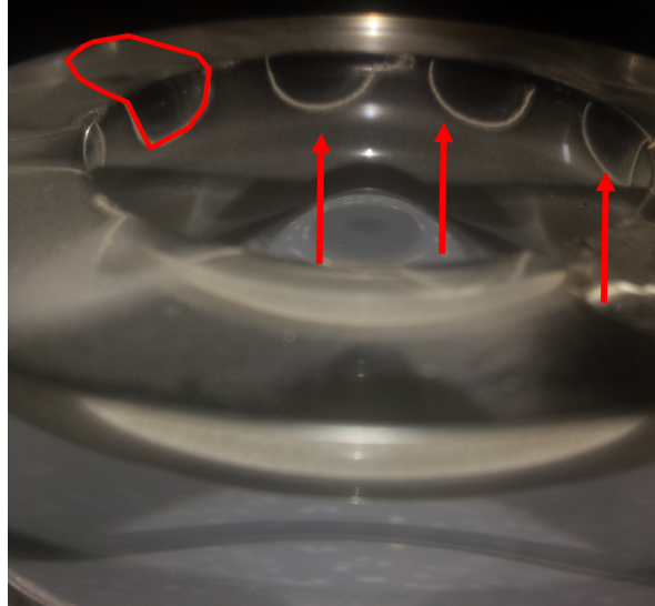
Figure 4.12. Sprays impacting on the piston lip.
