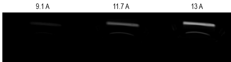
Figure 5.4. Lamp filament images for different electrical currents.
