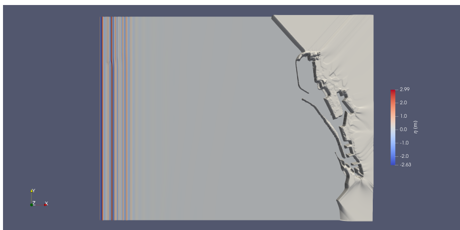
Figure 6.28: Simulation 3, wave propagation from the south-east direction into Barcelona harbor, H_s=5.0 m , T_p=10 s. Irregular waves generated from the left boundary. Refraction can be seen as waves propagate near shore.
