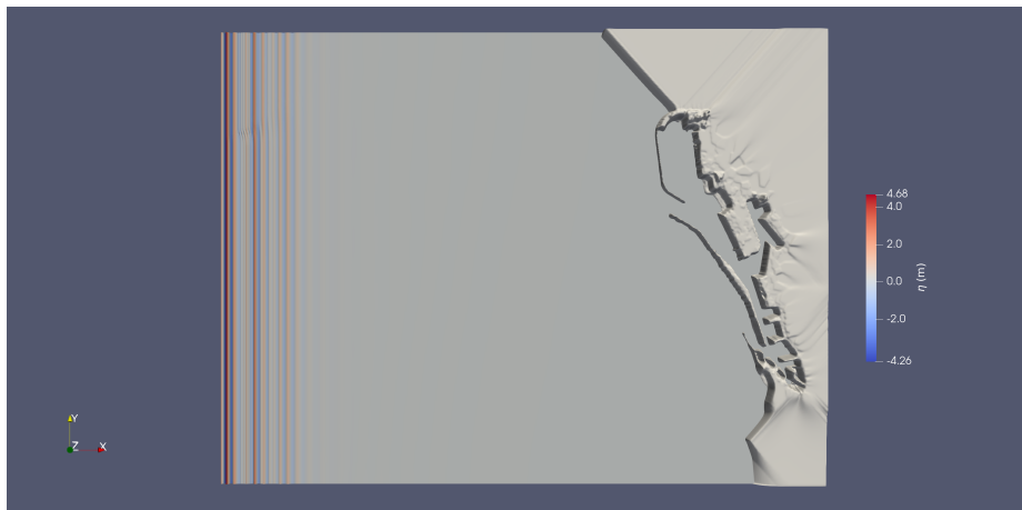
Figure 6.8: Simulation 1, wave propagation from the south-east direction into Barcelona harbor, H_s=5.21 m , T_p=12 s. Irregular waves generated from the left boundary. The effects of the changing bathymetry can be seen as waves are refracted while propagating towards shore.
