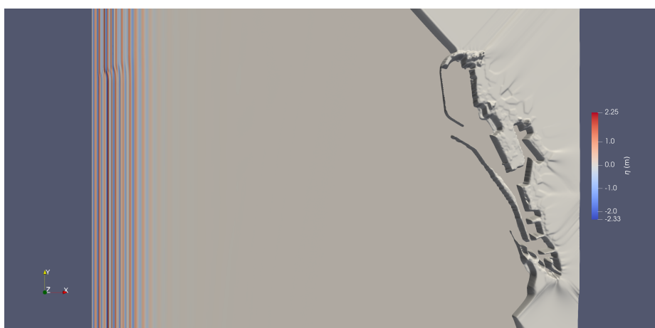
Figure 6.18: Simulation 1, wave propagation from the south-east direction into Barcelona harbor, H_s=4.5 m , T_p=11 s. Irregular waves generated from the left boundary.
