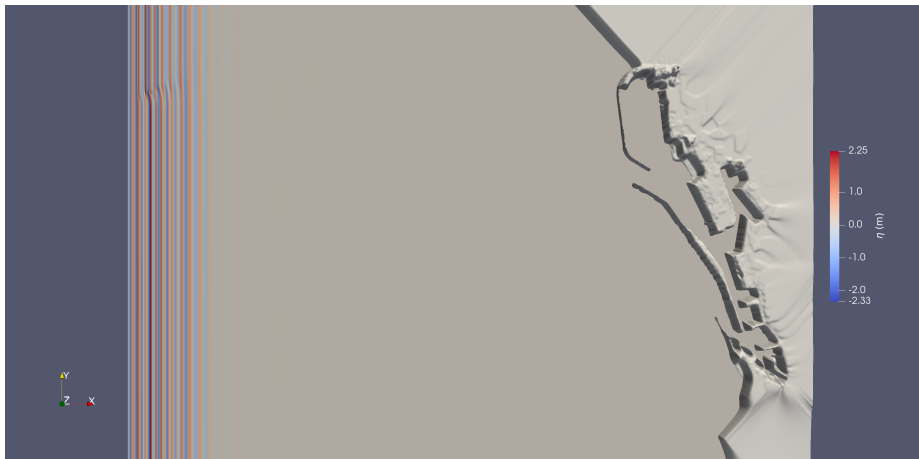
Figure 4.11: Simulation 2, wave propagation from the south-east direction into Barcelona harbor, H_s=4.5 m , T_p=11 s. Free Surface Reconstruction at t=450 s, generating waves at the left boundary.
