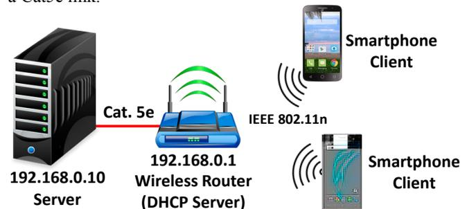
Figure 1. Scenario used during the test bench.
